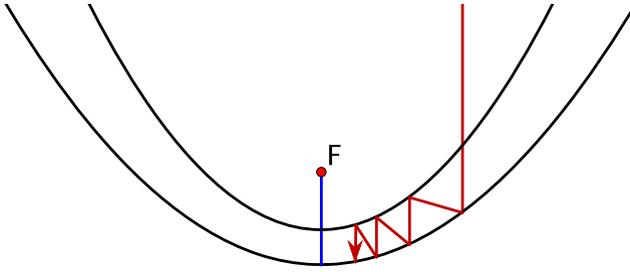
**Fig. 5** Trap for a parallel beam of light:  $F$  is the focus of the paraboloids
